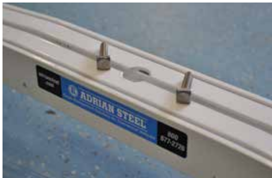
Crossbow with T-Slot and square-head bolts.
