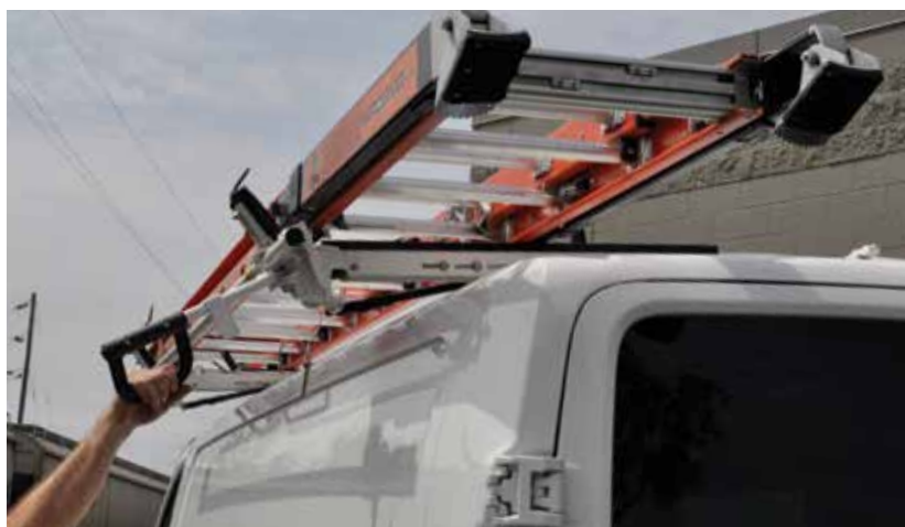
Pull to release the handle, swing out and down to lower ladder.
