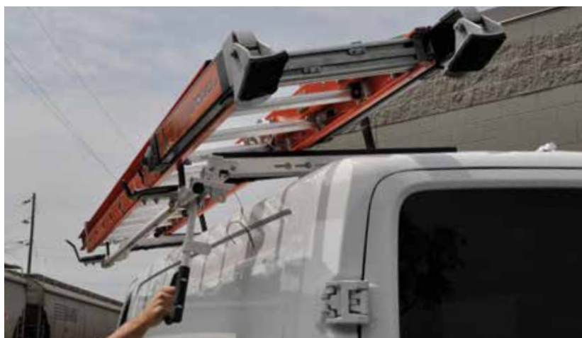
Pull to release the handle, swing out and down to lower ladder.
