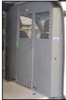
PA6-2 Door Kit converts M-Series fixed center panel into hinged door with keyed handle.
