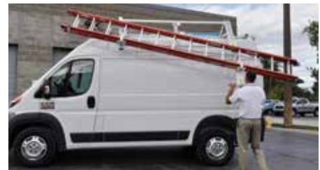
SECONDARY DROP & UNLOAD LADDER
