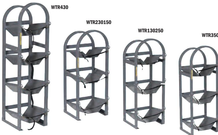
Vertically carry 30-lb. and 50-lb. refrigerant tanks securely in your van. Tank Racks can be installed for easy access from the side or rear van doors. Racks feature 14-gauge tubular steel frames welded for strength with sloped cradles and nylon straps. The optional **WTRTRAY** provides a storage area mounted on top of the welded tank racks.\* The tray can be mounted to any size tubular tank rack.
