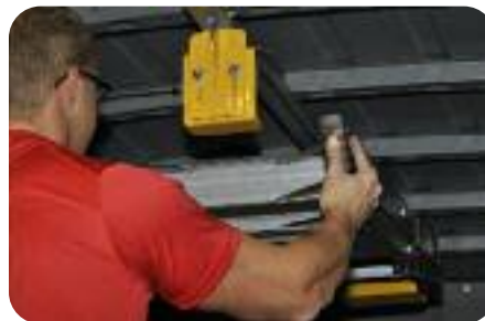
2 Walk the ladder back as the front clamp bracket glides on the track.
