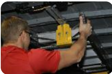
1 Simply press ladder inward to release rear ladder rung from the rear clamp bracket.
