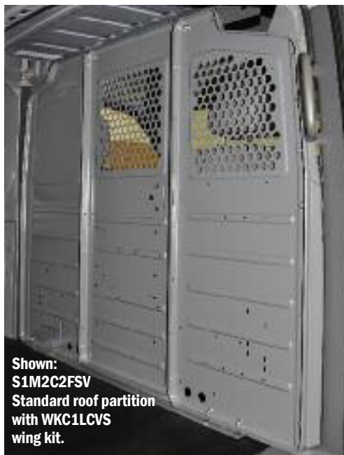
M1 Solid M2 Perforated Top Fixed center panels can be hinged as key- locking doors
