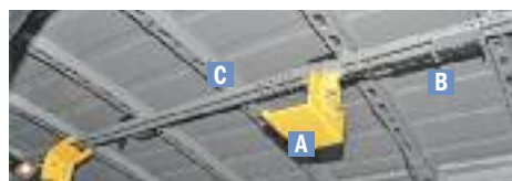
2 Walk the ladder back as the front clamp bracket glides on the track.
